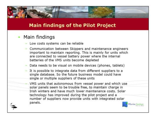
The project has used 3 different systems. Two requiring connection to vessel power and 1 with solar panels and independent of vessel power. The units vary in cost and depreciation. Low cost units can be reliable. Maintaining reporting of units which need vessel power has been the main problem as many Skippers withdraw power from the vessel during tie up or bad weather. This often requires units to be re-set remotely.
