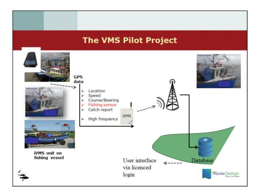
The Marine Institute have operated a pilot VMS project on vessels under 12m since 2014. All vessels fishing for razor clams are required to report position when fishing. Over 100 razor clam vessels have over the years been fitted with VMS units. A further 50 potters and netters on the south east and south west coasts joined the project in later years.
