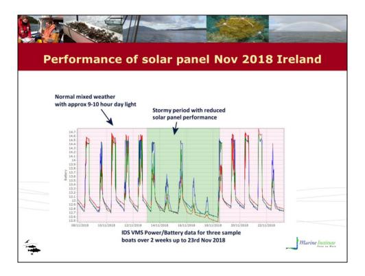
Solar panels maintain the internal battery of VMS units reporting at 10min frequency even during winter in Ireland
