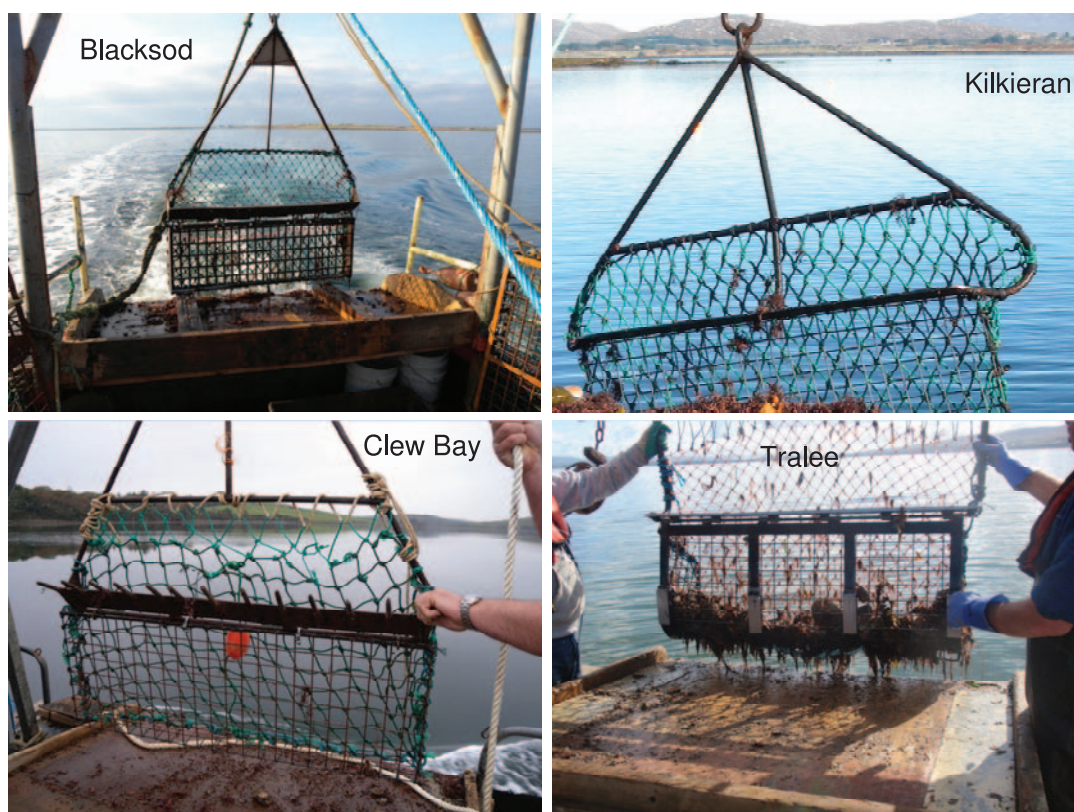
Figure 23. Dredges used on oyster surveys in Blacksod Bay, Kilkieran Bay, Clew Bay and Tralee Bay.
